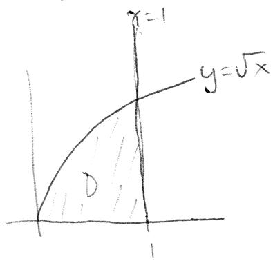
$$\text{Mass} = m = \int_0^1 \int_0^{\sqrt{x}} \rho(x, y) dy dx$$
